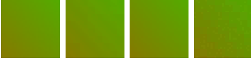
Fig. 2: Image gradient: Original, DXT1 (color bands, RMSE \approx 1.55 ), ftc1 (nearly no visible artifacts, RMSE \approx 0.94 ), ETC (color bands with jagged edges, RMSE \approx 3.63 )
