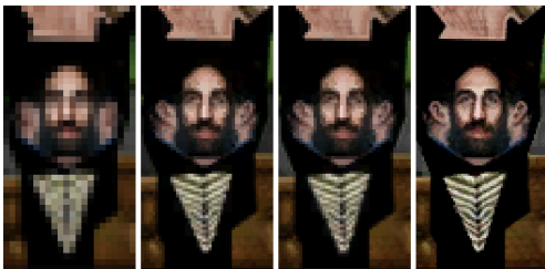
Fig. 6: Part of a RGBA texture from a computer game, rescaled to identical image size of 4 KB, transparent parts shown in grey: Uncompressed, DXT3, DXT5, ftc2.
