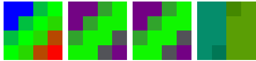
Fig. 7: Problematic block: Original, DXT1 (RMSE \approx 104.16 ), ftc1 (RMSE \approx 104.21 ), ETC (RMSE \approx 146.05 )
